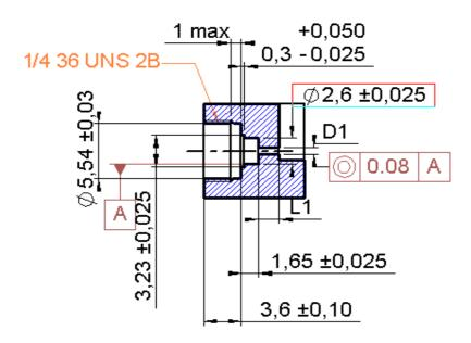
D1 and L1 dimensions have to be determined according to each application.
